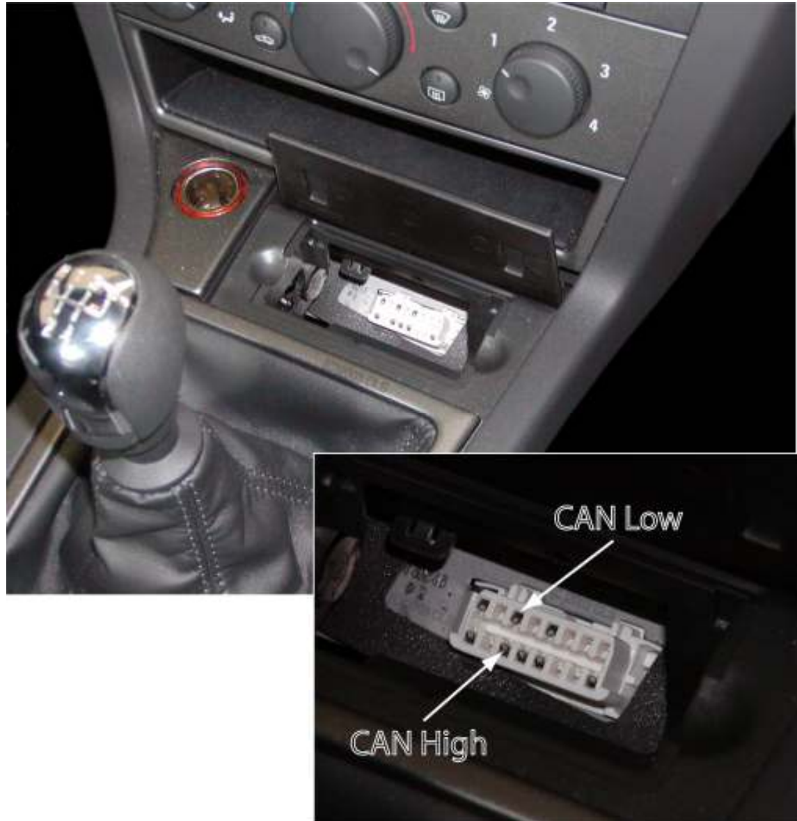
CAN Bus on diagnostic connector of Vectra Mk2
