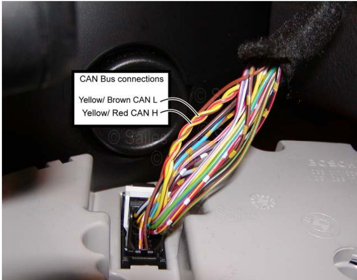
Picture from New Model BMW 3 series Wiring on rear of instrument cluster
